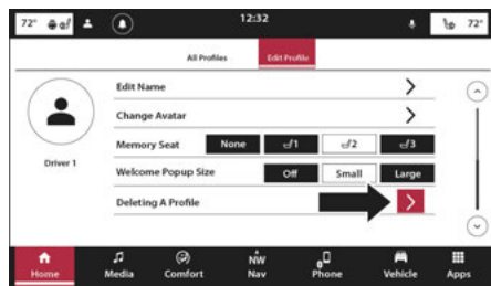
Uconnect 5/5 NAV With 10.1-inch Display Or 12-inch Display Profile Delete Button In Edit Profile
