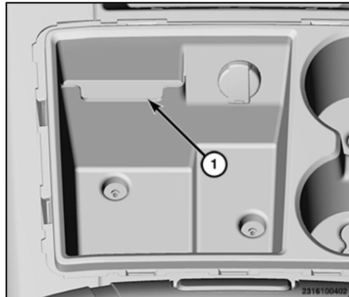
1. Using a trim stick [C-4755](#) or equivalent, release the rear retaining tab (2) of the front rubber mat (1).
