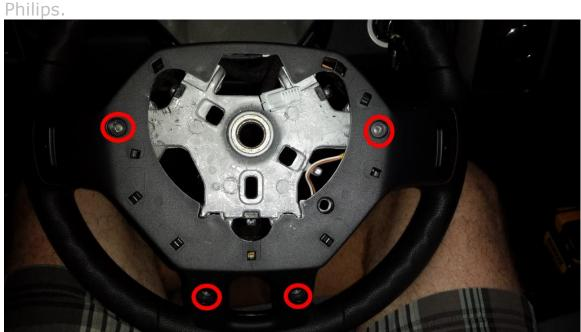
Inside the wheel the bottom 2 are Philips.
