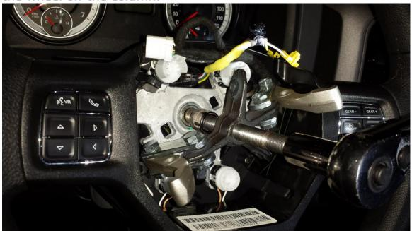
Be careful to not spin the airbag clockspring that holds the wheel electrical connection. Details below if you do turn it accidentally...
