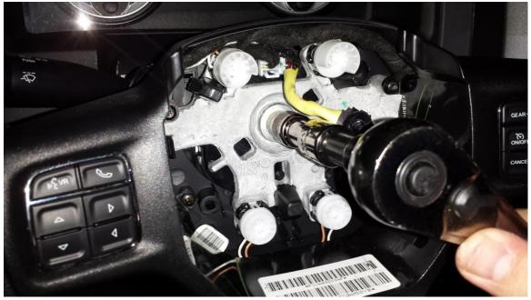
Step 6: Now its time to hook up the steering wheel puller and get the wheel off the column.
