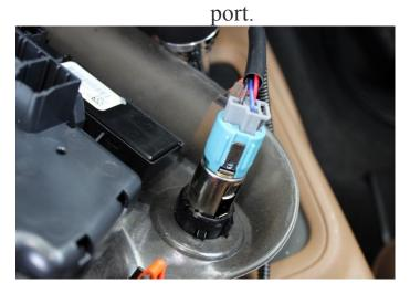
• Start the vehicle and wait 30 seconds. Insert the C-RVC programmer into the vehicle's OBDII port beneath the steering column. Once the programmer light turns green the installation is complete. Engage the vehicle into reverse to take advantage of your newly installed backup rear view
