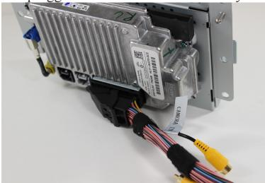
• Connect the camera's power (red) and ground (black) to the EZ DC 12v Accessory Kit. You can use basic crimpers to connect the wires. The EZ DC kit can then be plugged into the backside of any <u>switched/accessory</u> 12v cigarette lighter
