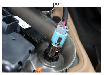
• Start the vehicle and wait 30 seconds. Insert the C-RVC programmer into the vehicle's OBDII port beneath the steering column. Once the programmer light turns green the installation is complete. Engage the vehicle into reverse to take advantage of your newly installed backup rear view camera!
