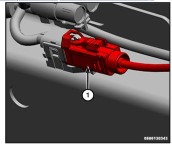
4. Remove the antenna mounting retainer (1).
