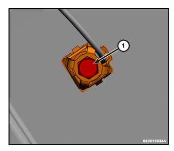
5. From inside the vehicle, using a flat bladed tool, press one of the two plastic retaining tabs on the antenna stud. Push up on one side of the antenna stud, press the other plastic retaining tab and remove the antenna from the sport bar.
