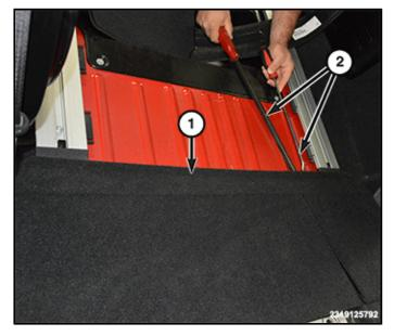
3. Remove the rear seat bolt and nuts (1), then the bracket (2).
