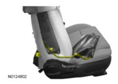
4. WARNING: Inspect the seat side air bag module cavity in the seat backrest foam pad for any foreign material. If any foreign material is found, remove it. Failure to follow these instructions may result in the seat side air bag module deploying incorrectly and increases the risk of serious personal injury or death in a crash.
