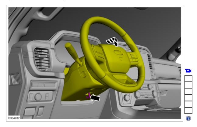
7. Release the tabs and disconnect the gap hider from the upper steering column shroud. Remove the General Equipment: Interior Trim Remover
