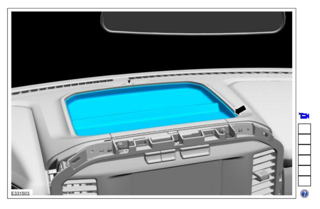
6. Remove the screws, release the clips and remove the upper instrument panel tray.
