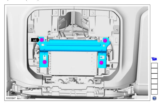
8. Remove the bolts, disconnect the electrical connectors and remove the <u>ACM</u> .
