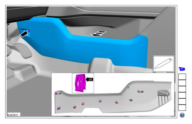
5. Release the clips and remove the floor console upper  $\underline{\mathsf{LH}}$  trim panel.
