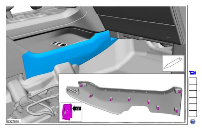
3. Release the clips and remove the floor console upper RH trim panel.
