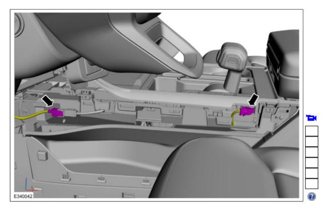
Remove the bolts and the floor console.
