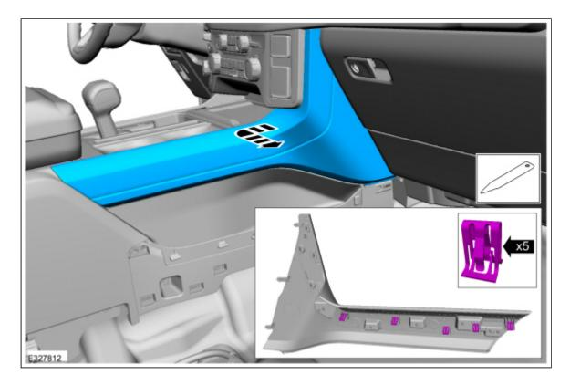
4. Release the clips and remove the floor console lower  $\underline{\mathsf{LH}}$  trim panel.
