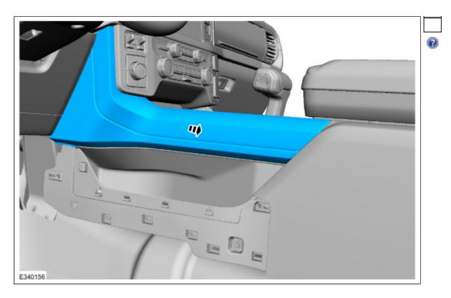
12. Install the floor console lower  $\underline{LH}$  trim panel and the screw. <code>Torque</code>: 22 lb.in (2.5 Nm)
