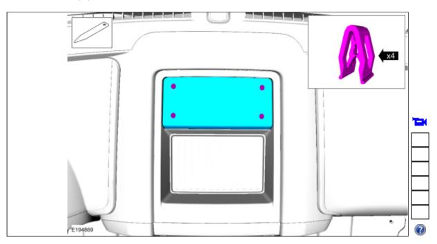
3. Remove the bolts, release the clips and remove upper instrument panel storage tray. *Torque*: 22 lb.in (2.5 Nm)
