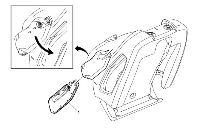
1. When installing the airbag module into the seat trim cover pouch, ensure there is no twisting of the pouch by fitting the module studs through the pouch holes for proper alignment and also make sure that the top of the module protrudes through the correct access hole. Call for technical support if you have any questions on this important step.
