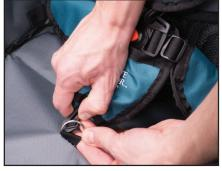
Ensure harness is secured to remaining three d-rings with the clips.
