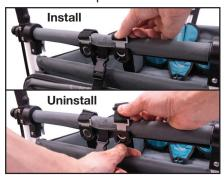
**To Install:** place shoulder straps over padded cross bar and push into slot. **To Uninstall:** press bottom tab with your thumb and pull out.
