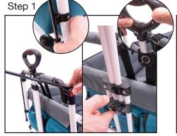
Rotate canopy rods to down position and secure in retaining clip. Release handle locking mechanism to fully retract handle and secure handle in handle retaining clip.
