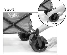
Rotate the front swivel wheels so they are both pointing outward, if they are not already. This is necessary for the wagon to fold compactly.
