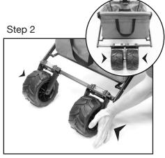
Push the rear wheels together and center on rear axle. Lightly tapping the wheel bracket with the heel of your palm can help. Beware of pinching.
