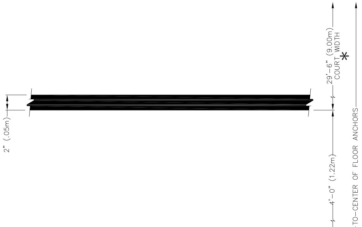
PLAN VIEW SHOWING PORTABLE VOLLEYBALL BASE AND FLOOR ANCHOR LAYOUT
