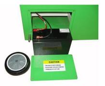
connected to the red terminal and black wire to the black terminal. Care must be taken to ensure you put the battery terminals to the top left side when you insert the battery into the cage.
