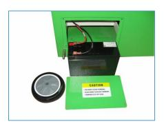
Please take extra care to ensure you put the battery terminals on the top left side when you insert the battery into the cage.
