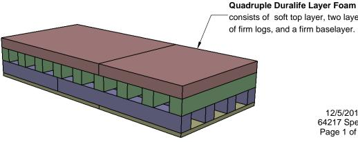
consists of soft top layer, two layers of firm logs, and a firm baselayer.
