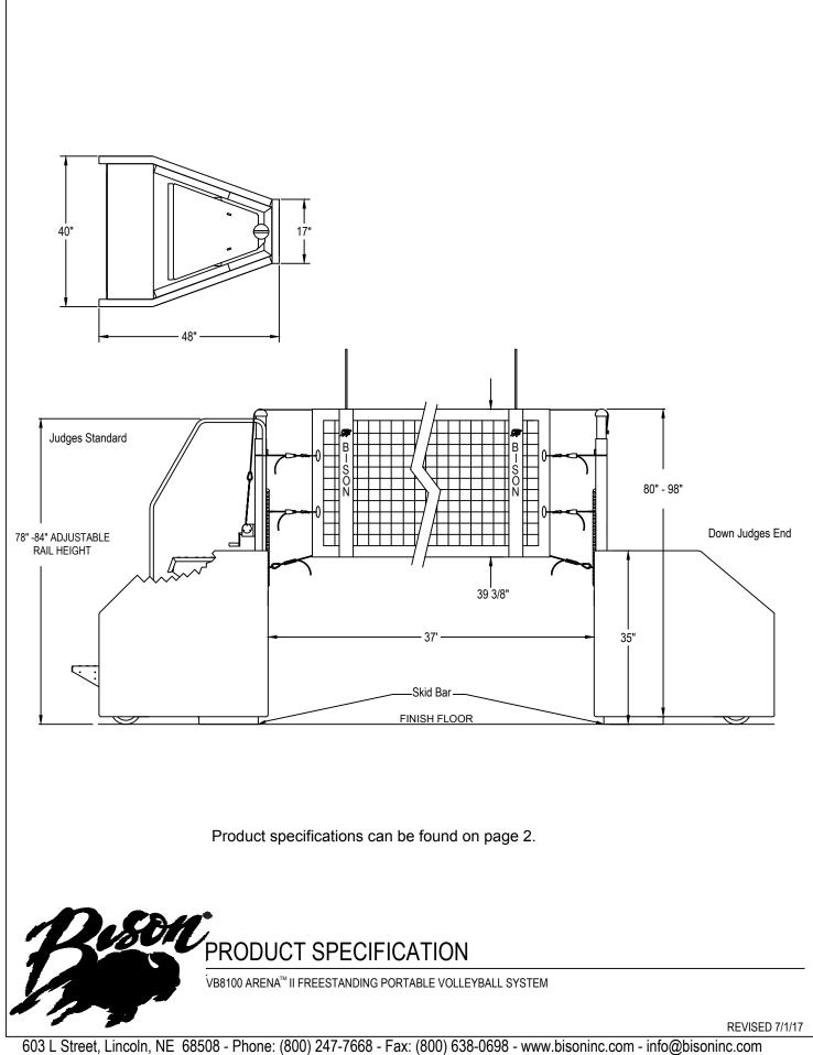
System shall be capable of providing elite competition level volleyball play without the use of additional loose ballast, floor hold downs or any wall or ceiling attachment. System shall be suitable for use on all floor systems designed for competition play including maple, molded square tile and synthetic and allow no less than 250# of net tensioning without movement of the bases.
