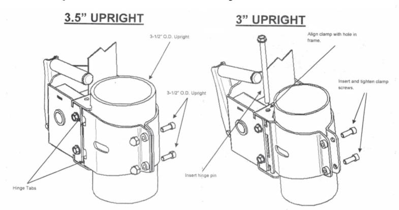
Slip the hinge tabs on the clamps into the winch slots on the winch housing.
