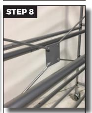
Attach center cross bar to rows two (2) and four (4) on each end pre-drilled center hole using wing nuts provided. Take note that it is easier to attach if all screws on shelf bars were left loose as noted in Step 7.
