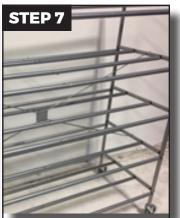
Attach shelf bars by starting at the bottom of each upright and attaching four (4) shelf bars per row using black plastic spacers and screws with lock washers. DO NOT TIGHTEN THE SCREWS! Leave slightly loose until all bars are attached.
