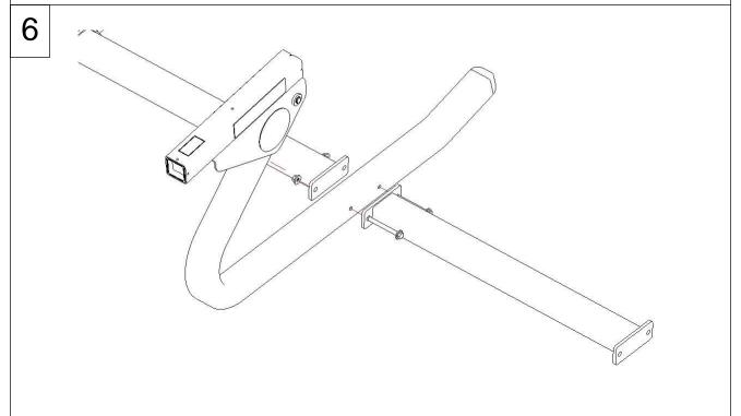
**For 2-7 man Lev Sleds:** Flip Lev Runner and Connecting Link upright. Bolt next Lev Runner (and Connecting Link, if applicable) onto connecting link from previous step. Repeat until Lev Sled is complete.
