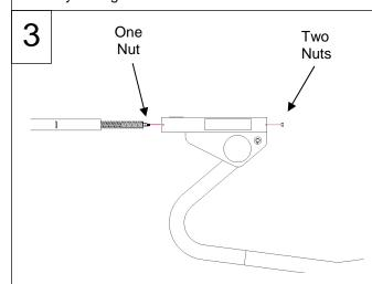
The Lev Ram Unit comes with (3) nuts on the threaded rod at the end of the spring. With (1) nut at the end of the spring, insert Ram Unit into sled head unit. Use the remaining (2) nuts to attach the ram unit to the sled. A screwdriver can be used to guide the threaded rod through the hole.
