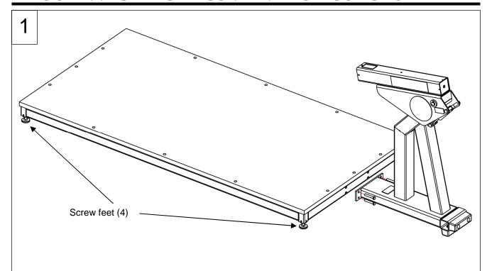
Use (4) bolts ½ x 3" to attach the Lev Unit to the Platform. Bolt head size is ¾". Adjust screw feet on the Platform to level it relative to the Lev Unit's height. Then install the Ram and Pad as outlined in steps 3 & 4 of the Lev Sled assembly on page 9.
