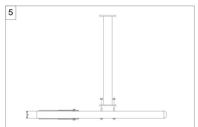
For 2-7 man Lev Sleds: Lay Lev Runner Sub Assembly on its side. Connect the runner to the connection link using (2) bolts and (2) nuts.
