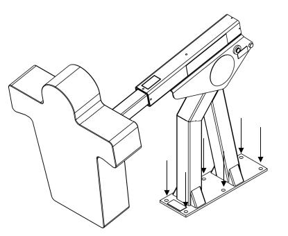
Consult a professional contractor, engineer, or building maintenance supervisor for hardware and procedures specific to installation in your building. For best results, mount to concrete. Mount securely using no less than six bolts. Maximum bolt size is ¾" diameter, grade 5; minimum bolt size is ½" diameter, grade 5. Install the Ram and Pad as outlined in steps 3 & 4 of the Lev Sled assembly on page 9.
