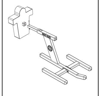
Use a fas-pin to fasten pad to the ram unit.
