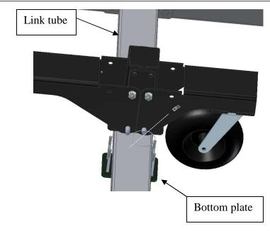
Attach wheel kit to center of link tube Insert 4 bolts into holes on bottom plate then put them thought top plate and tighten on 4 5/8 nuts
