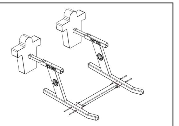
**For 2-7 man Lev Sleds:** See steps 3 & 4 for Ram Unit and Pad installation. To begin assembly lay Mod Sled runner on its side. Connect the runner to the connection link and then stand runner upright to connect the next sled runner. Hardware used for the Connection Links is (4) 5/8" x 6" bolts, (4) 5/8" nuts, and (8) 5/8" washers per Mod Sled Runner.
