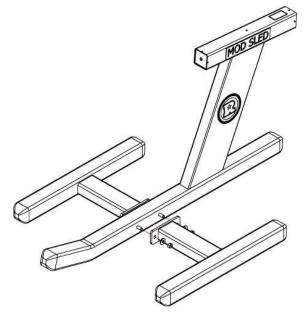
Fit second outrigger over the bolts and secure with (2) more 5/8" washers and (2) 5/8" nuts.
