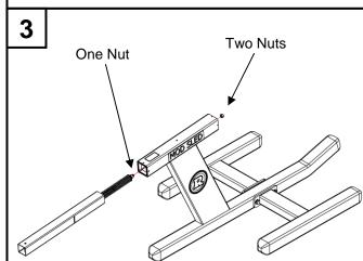
The Mod Ram Unit comes with (3) nuts on the threaded rod at the end of the spring. Remove (2) nuts to use later. Install the Mod Ram Unit by inserting it spring side first into the Ram Outer Tube. The threaded rod on the end of the spring fits through a hole at the back of the head unit. A screwdriver can be used to guide the threaded rod through the hole. Use the nuts you removed earlier to secure the ram in place.
