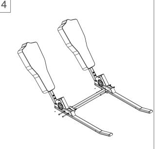
For 2-7 man Powerline Sleds: Use the (2) 5/8" x 6" bolts, (2) 5/8" nuts, and (4) 5/8" washers to connect each PL runner to connection link. Repeat steps 3 & 4 for each additional unit installed
