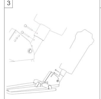
Insert the pad tube into the PL Sub Assembly with the graphics of the pad facing toward the training area. Use fas-pins to fasten the pad to the PL Runner.
