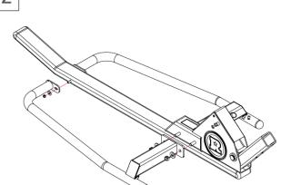
Fit second outrigger over the bolts and secure with (2) more 5/8" washers, (2) 5/8" nuts, (1) 3/8" washer and (1) 3/8" nut.
