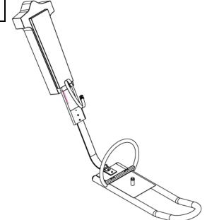
Attach the Tackle Sled Pad Frame to the leaf spring with (2) ½" x 1 ½" bolts and (2) ½" nuts.
