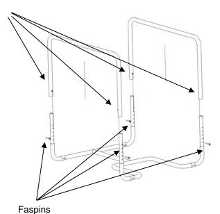
Flip parts from Step 1 upside down. Insert fas-pins into desired height positions. Make sure all pins are at an equal height. Place (2) Runners onto elbows as shown. Flip over Chute and make sure fas-pins are resting against the runner, tighten (4) 3/8" bolts.
