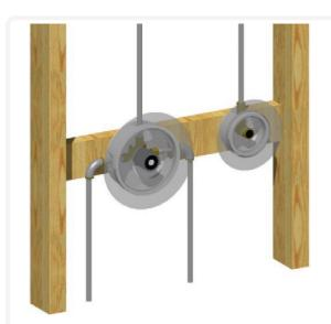
Remove the manufacturer's recommended size access hole for the mixer from the large flange. Remove a 30mm hole from the small flange. Apply a bead of sealant to the channel on the flanges and firmly push onto the cups.
