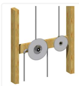
Remove identical holes from the wall lining to match. Apply the remainder of the sealant to the outside of the flanges.
