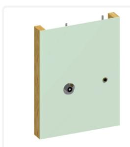
Fix the wall lining. Distribute excess sealant over exposed wall lining core in the holes.
