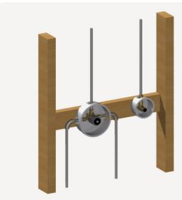
Fix cups to the frame so that they finish flush with the wall stud. Plumb out the fittings.
