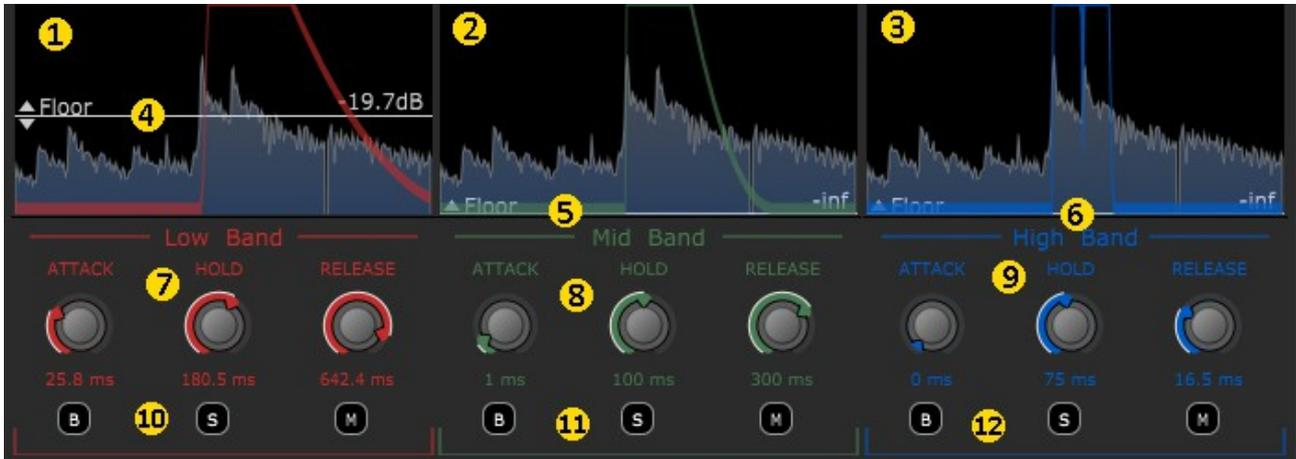
1. Low Band windows showing the Low Band waveform and Low Band gate envelope
