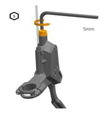
2. Insert the hose into brake lever hole until the hose touch the bottom surface, insert compression fitting, tighten the compression nut.
