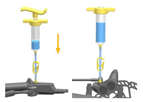
5.3. Hold the syringe at the caliper vertically while slowly pressing down on the syringe plunger at the caliper, push the oil located at the caliper towards the brake lever.
