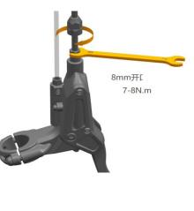
2. Insert the hose into brake lever hole until the hose touch the bottom surface, insert compression fitting, tighten the compression nut.
