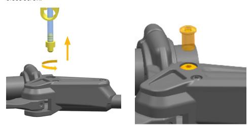
5.7. Clean any mineral brake oil that drips from the bleed port with isopropyl alcohol and a shop towel. Spray isopropyl alcohol on the brake lever and caliper and clean them with a shop towel.
