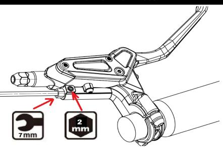
Use 2mm Allen key release the M4 lock screw, rotate the adjust bolt clockwise or counterclock wise with 7mm spanner until the power off switch can work properly when press lever blade for 10~15mm. Tighten the M4 lock screw with 1.5Nm torque.
