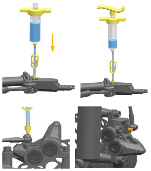
5.5. Open the valve or clamp on the syringe at the lever. Squeeze and release the lever blade 3-5 times.
