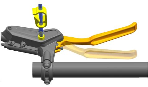
5.6. Close the valve or clamp on the syringe at the brake lever. Remove the syringe at the lever from the leed port. Install the bleed screw. Use a T10 TORX to tighten the bleed screw.
