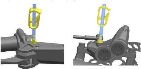
5.2. Hold the syringe vertically. Gently push the plunger down, stopping before air enters the hose tube. Oil will fill the syringe at the brake caliper. If the oil in the syringe at the caliper is discolored, continue to push all the oil out of the system. Restart the bleed procedure with new fluid in both Syringes.
