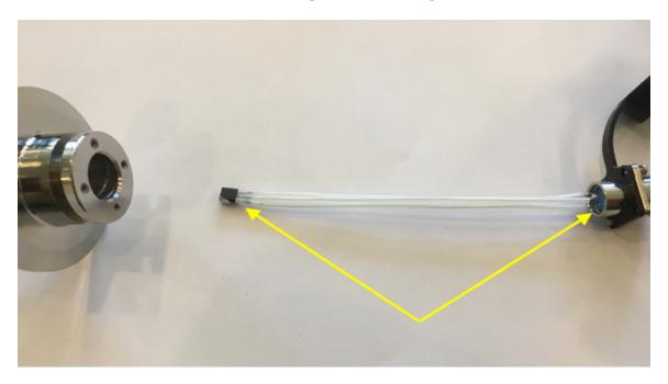
4. The sensor is a small computer chip and should be treated carefully as one would a computer (ie. don't be rough with it and don't place it near a magnet).
