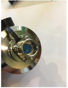
2. Loosen the four screws with a small Phillips screwdriver.
