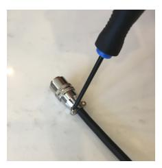
2. With your index finger pushing down on the white (blue on older models) portion of the connector, and two fingers of one hand gripping the collar (to hold the top portion secure), with the other hand unscrew the collar (lower portion) from the connector.
