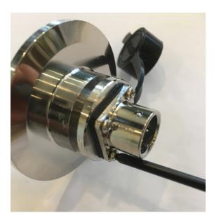
3. Gently slide the sensor out and inspect the wire joints at the connector end and at the sensor end. An unconnected wire will cause the sensor to malfunction. The compound on the sensor is heat transfer compound and should not be removed as it facilitates faster temperature reading.
