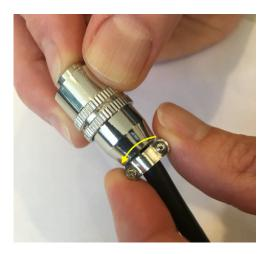
3. Move the collar down the cable and inspect the soldered cable joints. They should be intact. A broken connection will be easy to spot as an unconnected wire. If the wires are detached and need to be resoldered, the correct pin assignment can be confirmed by looking at the other end of the cable and matching the color of each wire to the number of the pin. The factory default is pin 1 is for the yellow ground wire, pin 2 is for the black positive wire, and pin 3 is for the red signal wire.
