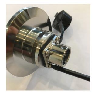
3. Gently slide the sensor out and inspect the wire joints at the connector end and at the sensor end. An unconnected wire will cause the sensor to malfunction. The compound on the sensor is heat transfer compound and should not be removed as it facilitates faster temperature reading.
