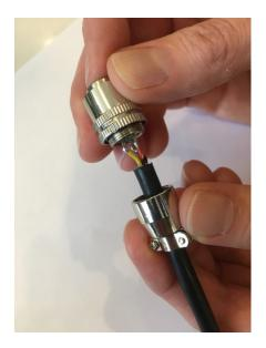
4. Reattach the collar with the above steps in the reverse order. Ensure that the cable and cord end are not twisted when reinstalling as this can put tension on the solders; only the collar should turn. And when retightening the cord grip on the collar, ensure that the cable is snug and cannot move under the cord grip. Over time the cable jacket might age and
