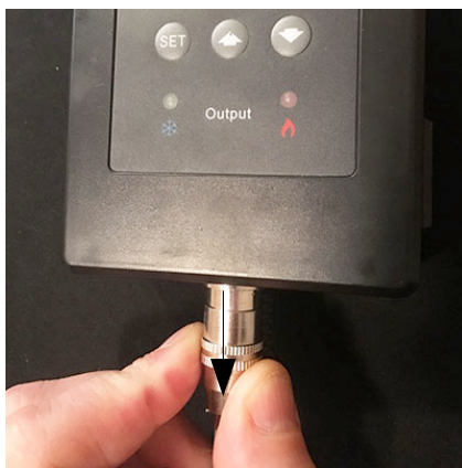
Figure 4. Pull the spring loaded collar to remove the sensor cable.
