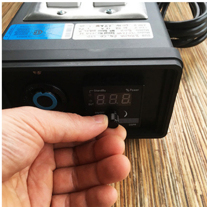
Figure 37: Knob controls percentage of power output
