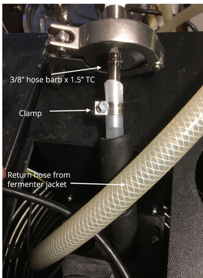
Figure 46: Connect the chiller to water circulation hoses
