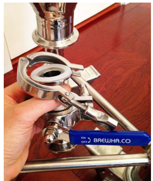
Figure 15: Bottom (dump) valve
