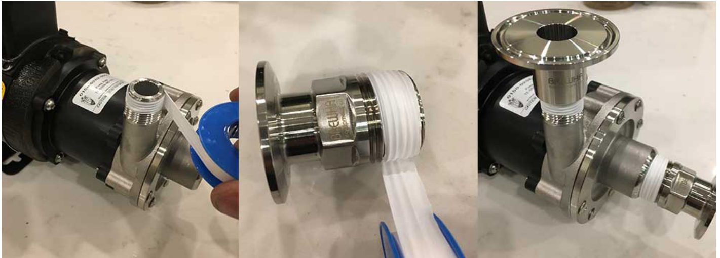
Figure 27: Adding sealing tape to threads
