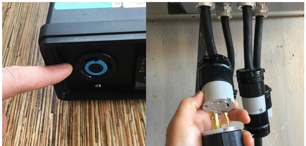
Figure 36: Connecting heater extension to box
