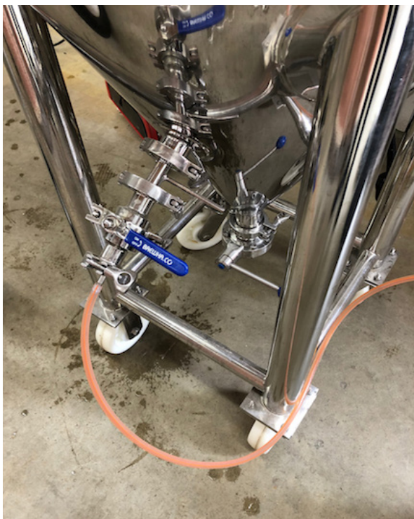
Figure 17: Racking port with serving hose
