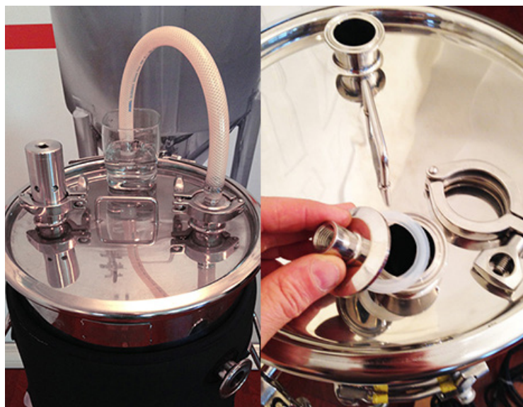
Figure 22: Attaching blow-off hose or gas in connection
