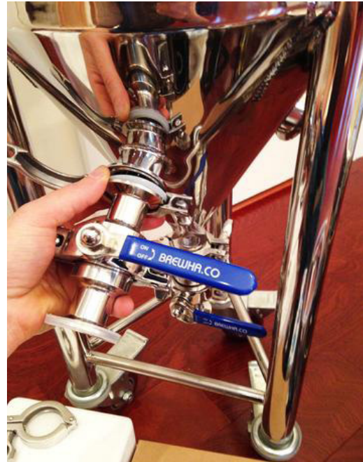
Figure 16: Side racking valve
