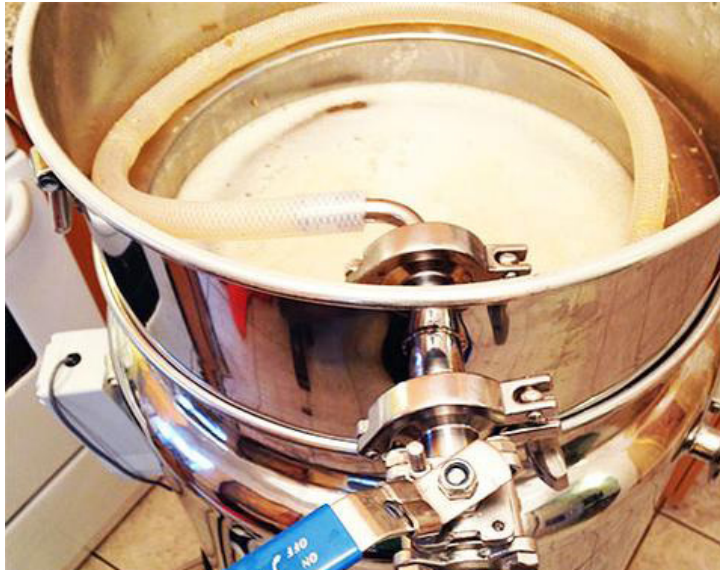
Figure 28: Valve attached to inlet port on Mash Colander
