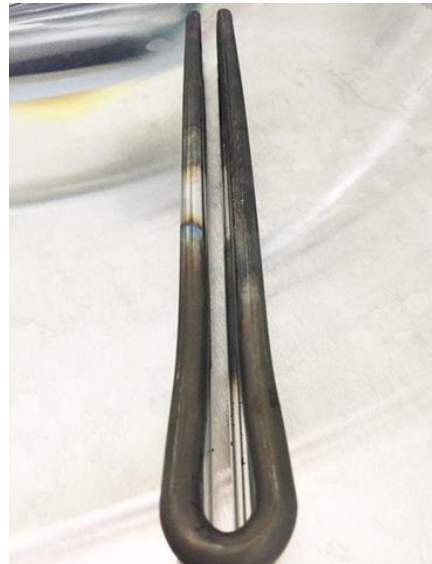
Figure 3: Internal heater failure
