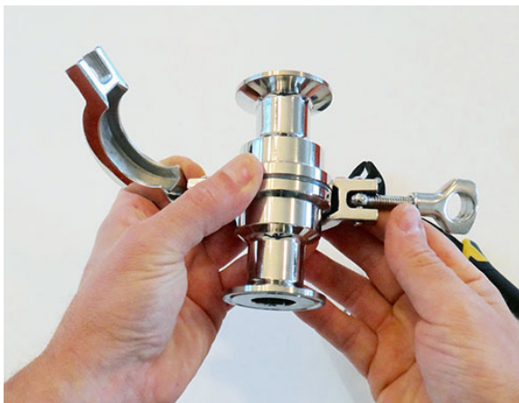
Figure 30: Removing the sanitary clamp
