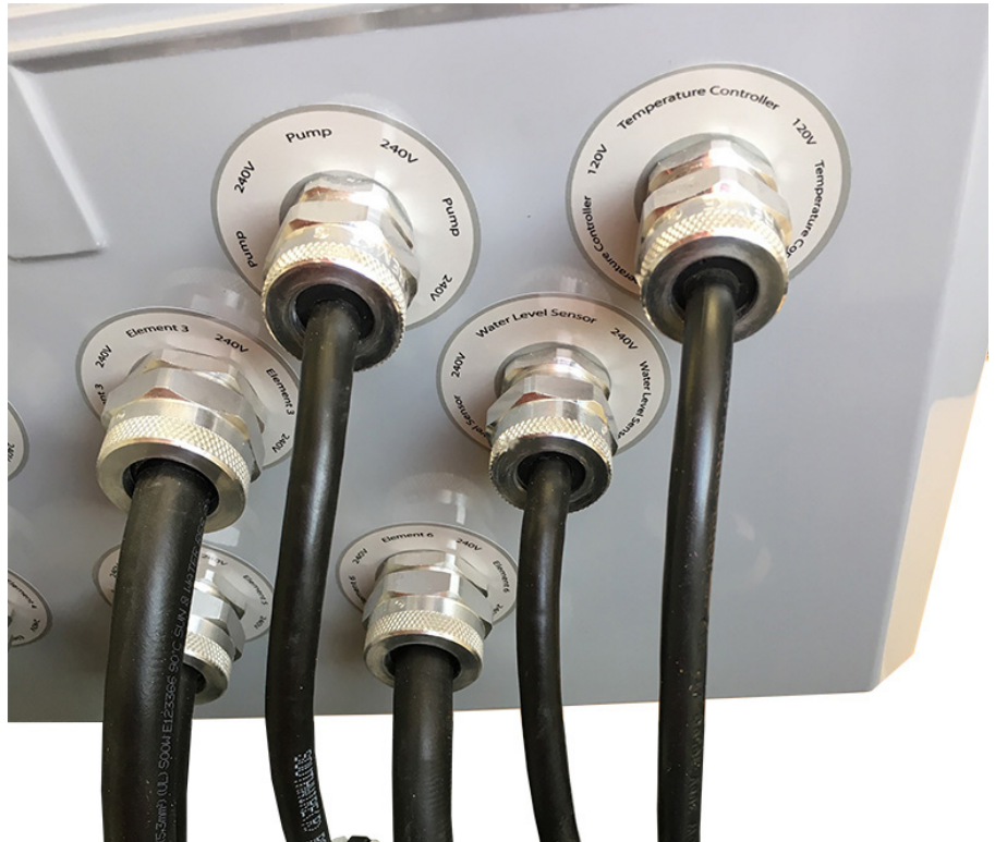
Figure 38: Additional outputs on the bottom of the controller
