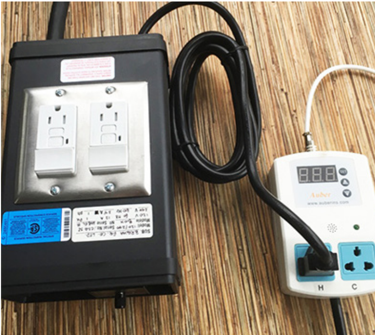
Figure 35: Connecting the contactor cord to the ETC
