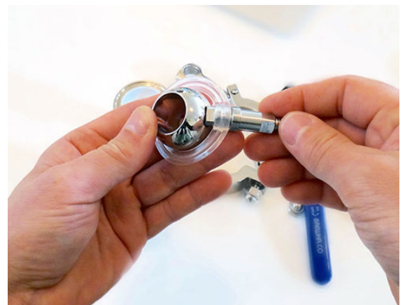
Figure 31: Removing the ball stem
