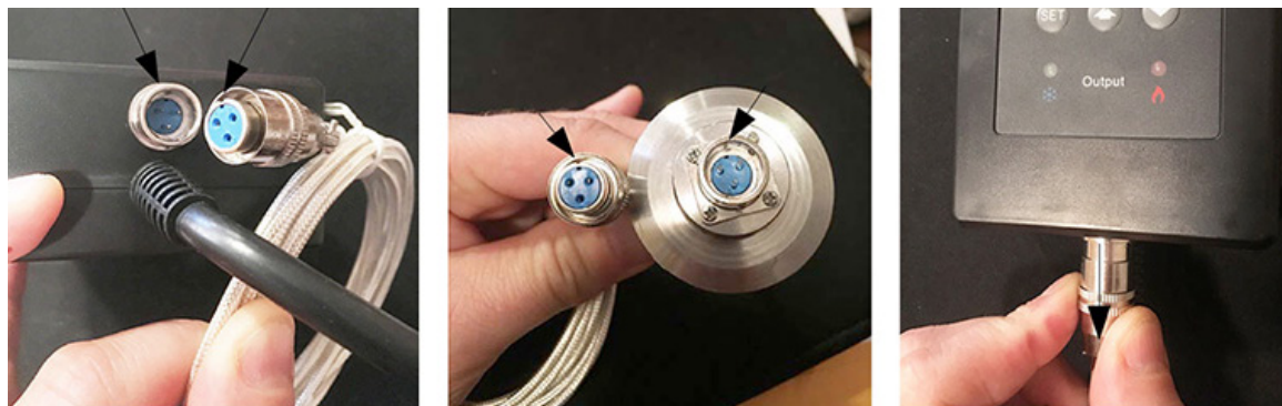
Figure 42: Attaching the sensor cable to the ETC
