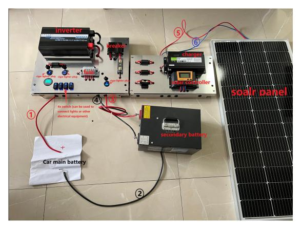
No.1 red wire connected to the positive electrode of the car main battery. No.2 black wire is used for connecting the negative electrode of the car main battery to the negative electrode of the secondary battery.
