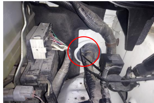
5) Connect positive pole line to the left side of the car
