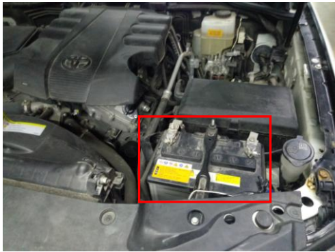
1) Open engine compartment and find the battery
