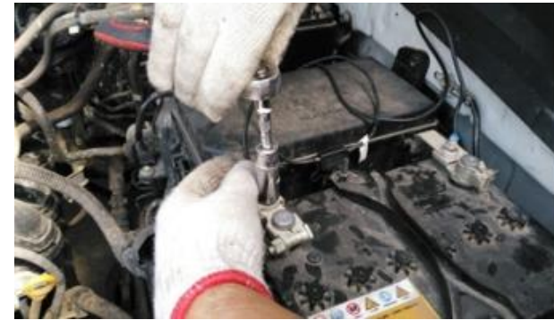
3) connect positive pole of a battery CAUTION!: Tighten battery screw very tight! If loose, may get damage to the car.
