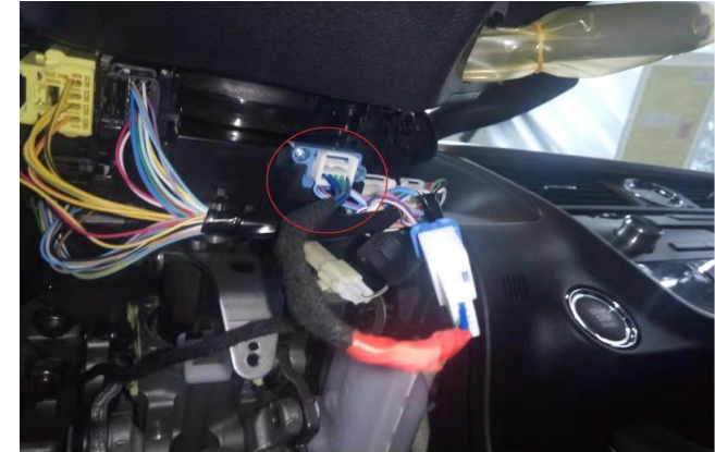
9) Directly insert OBD in the diagnostic interface OBD of original vehicle in this place
