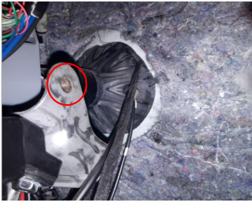
7) Find the left original M6 screw hole
