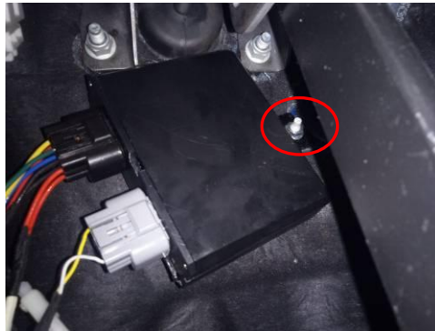
7) fixing ECU as above picture
