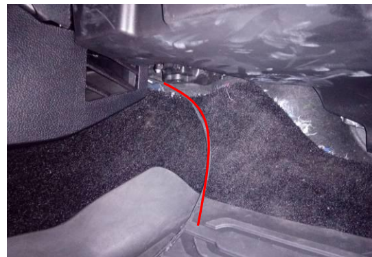
11) another motor line to co-drive side
