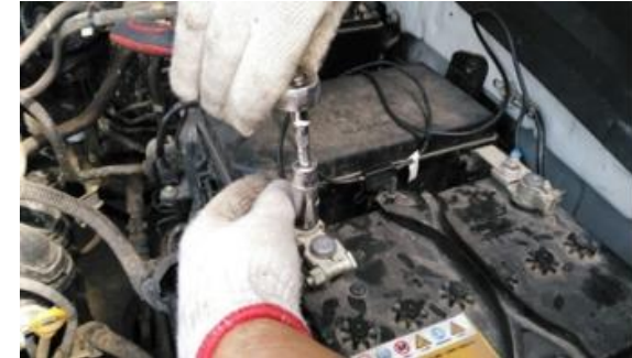
3) Caution: Tighten battery screw very tight! If loose, may get damage to the car
