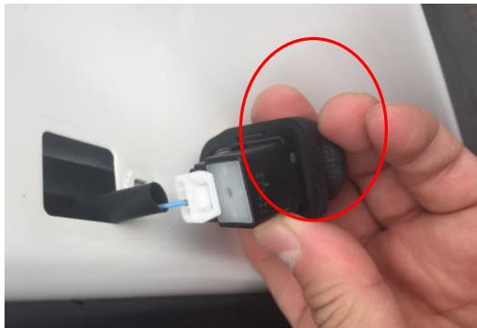
11) plug in the connector with door switch
