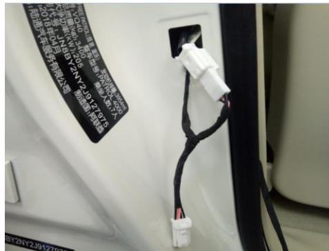
12) connect with door switch and recover it
