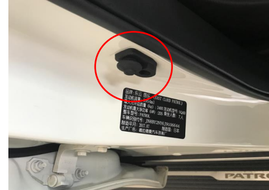
9) take out the door switch connector
