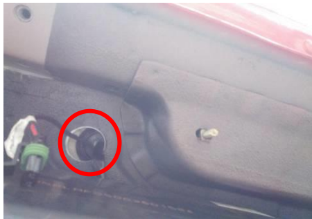
9) motor line from this hole to cabin
