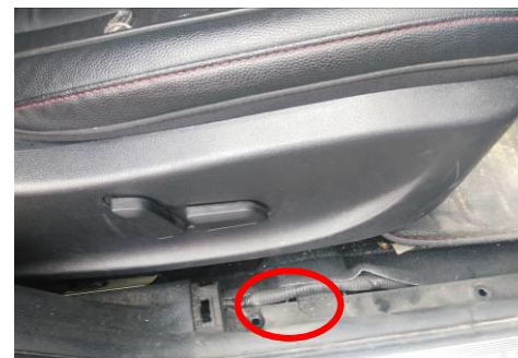
7) right motor line from above position from chassis to cabin, under seat
