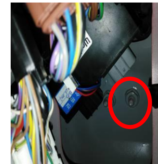
6) ECU fixing as above by screw
