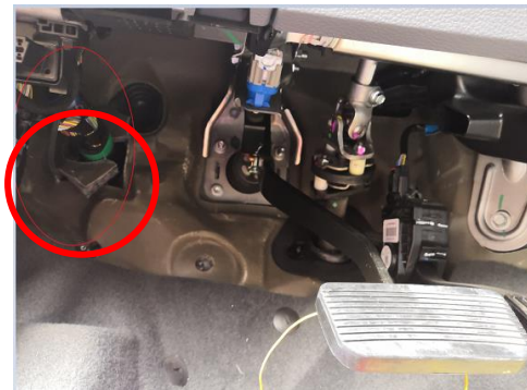
LHD:Connector is at left of LF Position as above picture RHD:Connector is at right of RF
