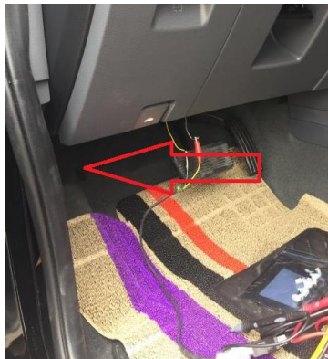
LHD:Connector is at left of LF Position as above picture RHD:Connector is at right of RF
