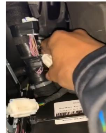
Plug it with upper one by our connector and insert it back.
