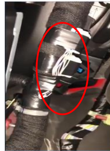
Connector covered by tape along with wiring
