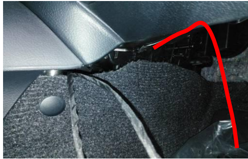
7) left motor wire from this position to left side
