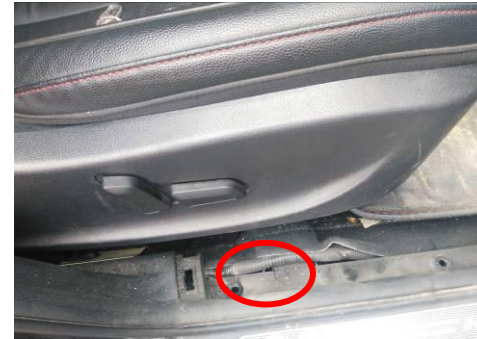
9) right motor line from above position from chassis to cabin, under seat
