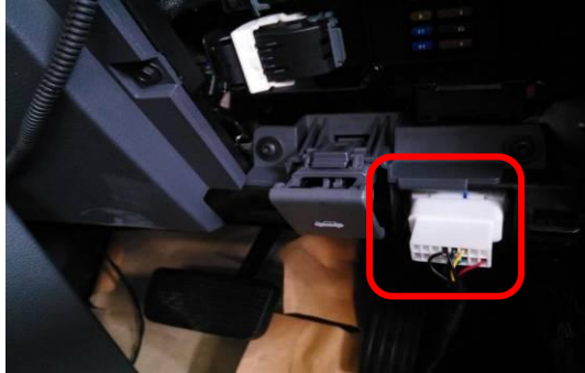
8) connect OBD as above picture
