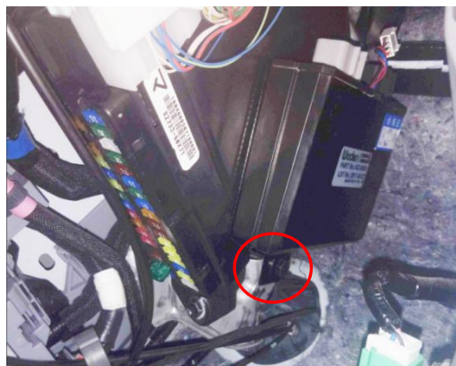
8) Fix with M6 screws
