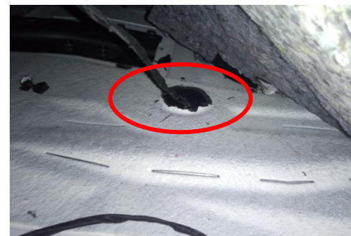
12) Lift the carpet on the right, Connect the right motor line to the chassis
