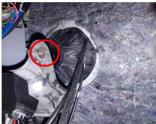
7) Find the left original M6 screw hole
