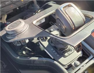
9. Release the vehicle wiring harness from the auto start-stop switch assembly. If you have difficulty releasing the connector, try removing the switch assembly through the top by releasing the side retaining clips.
