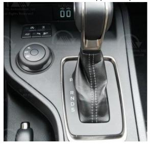
13. Reconnect the electrical connectors on the lower center stack trim panel, place it into position and reinstall the 7mm bolts in each side.
