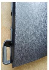
5. Remove the finish panel to the lower right side of the HVAC controls by gripping the edge with a firm grip and gently increasing pressure to release the 6 fasteners. There is an alignment dowel molded into the plastic in the upper left corner, so be sure to only pull straight back in this area.
