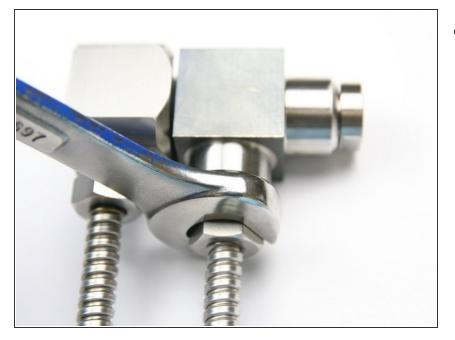
Tighten the high-pressure gland nut into the swivel housing with a 5/8" wrench.
