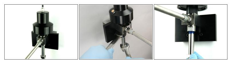
(i) The valve kit components can be replaced with the valve body in the mounting collar.
