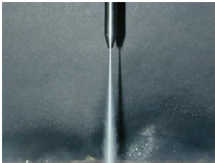
Good abrasivejet stream
