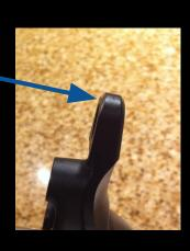
2. Chamfer should be ~45 degrees and should NOT extend to the bolt hole (~1/2 way from tip to bolt hole)
